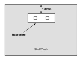
Once the base plate has been positioned, mark two holes through the bolt apertures. Drill through the desk at the marked positions using an 8mm drill bit.
